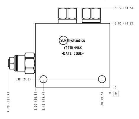
This valve assembly provides overrunning load-control and load-port relief protection and includes a load sense shuttle for brake release. Connecting the T port is optional and will supply make-up oil and may flush hot dirty oil out of the
