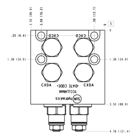
This valve assembly provides overrunning load-control, load-port relief protection, supplies make-up oil, and flushes hot dirty oil out of the actuator. All oil coming out of the actuator returns to tank through port T.
