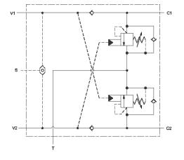
This valve assembly provides overrunning load-control, load-port relief protection, supplies make-up oil, and flushes hot dirty oil out of the actuator and includes a load sense shuttle for brake release. All oil coming out of the actuator returns to tank through port T.
