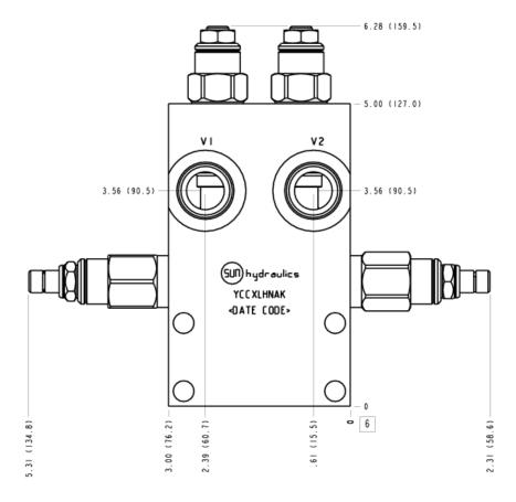
This assembly provides 2 functions, a) dual cross-pilot load holding between motor ports M1 and M2, and b) cross-port relief protection between ports M1 and M2.
