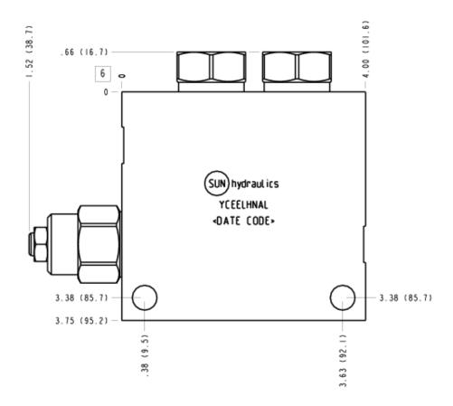
This valve assembly provides overrunning load-control and load-port relief protection, Connecting the T port is optional and will supply make-up oil and may flush hot dirty oil out of the actuator. Oil coming out of the actuator may return to tank through either port T or the directional valve.
