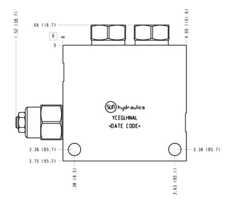
This valve assembly provides overrunning load-control and load-port relief protection and includes a load sense shuttle for brake release. Connecting the T port is optional and will supply make-up oil and may flush hot dirty oil out of the actuator. Oil coming out of the actuator may return to tank through either port T or the directional valve.
