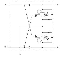
This valve assembly provides overrunning load-control and load-port relief protection and includes a load sense shuttle for brake release. Connecting the T port is optional and will supply make-up oil and may flush hot dirty oil out of the actuator. Oil coming out of the actuator may return to tank through either port T or the directional valve.
