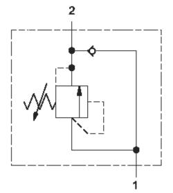
This assembly provides 2 functions. It relieves pressure from (port 1) to (port 2) when pressure at port 1 exceeds the setting of the valve and incorporates a check valve that allows reverse flow from port 2 to port 1.
