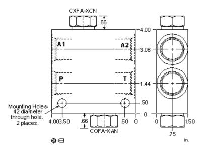
This assembly will automatically discharge an accumulator through a 0.125 inch orifice whenever the pump is shut off. Whenever the pump is started, the pilot-to-close check valve closes, blocking the discharge path back to tank. The standard check valve prevents oil in the accumulator from back-flowing through the pump.
