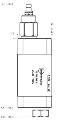
This assembly consists of direct-acting relief cartridge which is normally closed, pressure-limiting valve and also includes a check valve that allows reverse free flow.
