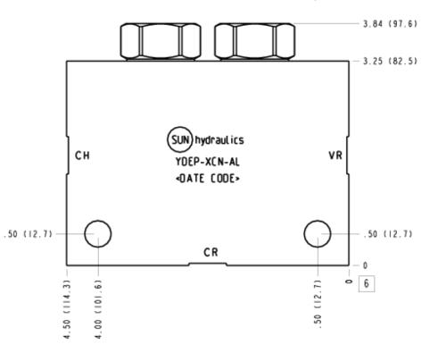
The full time regenerative valve assembly allows a double-acting, single rod cylinder to be extended more rapidly using the same pump flow. To achieve this, oil from the rod end of the cylinder (CR) is added to the pump flow to the blind end (CH), increasing the rate of extension. VR is the connection to the retract side of the directional valve.
