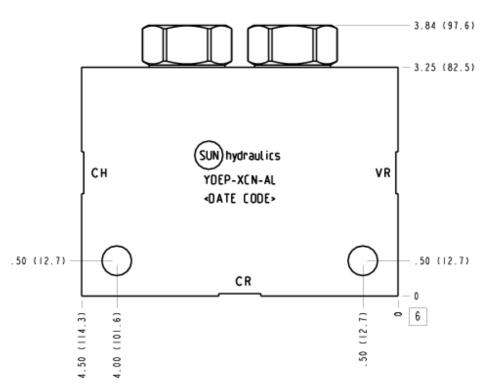
The full time regenerative valve assembly allows a double-acting, single rod cylinder to be extended more rapidly using the same pump flow. To achieve this, oil from the rod end of the cylinder (CR) is added to the pump flow to the blind end (CH), increasing the rate of extension. VR is the connection to the retract side of the directional valve.
