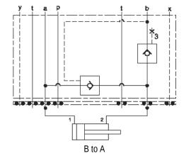
The full time regenerative valve assembly allows a double-acting, single rod cylinder to be extended more rapidly using the same pump flow. To achieve this, oil from the rod end of the cylinder is added to the flow to the blind end, increasing the rate of extension.
