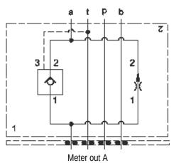
**NOTES:** • *Important:* Carefully consider the maximum system pressure. The pressure rating of the manifold is dependent on the manifold material, with the port type/size a secondary consideration. Manifolds constructed of aluminum are not rated for pressures higher than 3000 psi (210 bar), regardless of the port type/size specified.
