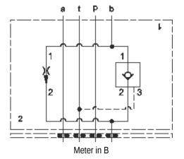
This assembly consists of a fixed-orifice, pressure-compensated flow control valve which provides precise flow regulation for meter-in or meter-out applications where there may be wide pressure fluctuations. The flow setting is specified by the user and is set at the factory.
