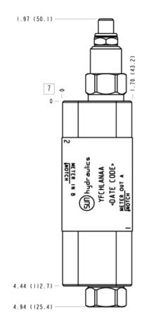
This assembly consists of a fully-adjustable, pressure-compensated flow control with reverse-flow check which provides precise flow regulation for meter-in or meter-out applications where there may be wide pressure fluctuations. It is infinitely adjustable from nearly closed up to the maximum flow. An integral high-capacity check valve provides unrestricted flow in the reverse direction. The rapid or feed rate is selected by a vented, pilot-to-open check valve with an external pilot port.
