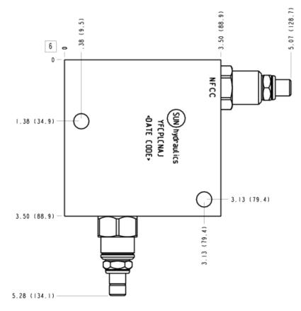
This assembly consists of a three-port normally closed modulating element with relief which provides two functions when combined with an external orifice. The mainstage is a bypass compensator that controls a priority flow into the circuit, determined by the orifice created by the needle valve. Input flow in excess of the priority flow is bypassed to tank (port T). If the inlet (port P) pressure rises to the valve setting, the valve operates as a normal relief valve.
