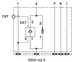
**NOTES:** • The external 1/4 NPTF pilot port is part of the pilot to open check cartridge.
