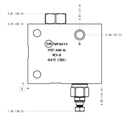
This assembly consists of a bypass/restrictive, fixed-orifice, priority flow control which takes an input flow at port P and uses it to satisfy the priority flow at port CF. If the input flow exceeds the priority flow requirement, the excess is bypassed out port EF. The bypass flow may be used in a secondary circuit. The relief valve protects the controlled flow from over-pressurization, relieving excess flow out of port T.
