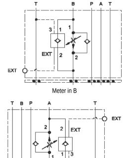
This assembly consists of a fully-adjustable, pressure-compensated flow control with reverse-flow check which provides precise flow regulation for meter-in or meter-out applications where there may be wide pressure fluctuations. It is infinitely adjustable from nearly closed up to the maximum flow. An integral high-capacity check valve provides unrestricted flow in the reverse direction. The rapid or feed rate is selected by a vented, pilot-to-open check valve with an external pilot port.
