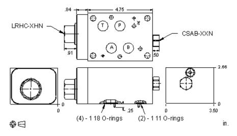
This valve assembly consists of a normally-closed bypass style compensator on the P port and a shuttle that senses pressure from the higher of the 2 work ports. Its purpose is to provide a relatively constant pressure drop across the directional valve thus isolating the directional valve spool from high flow forces. This is accomplished by bypassing the excess oil to the T port. The constant drop creates a pressure compensated flow control out of the directional valve.
