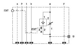
This assembly consists of a needle valve which is a fully-adjustable orifice used to regulate flow. It is infinitely adjustable from fully closed up to the maximum orifice diameter. It is not pressure-compensated. It may be used as a flow control or as a shutoff valve. The rapid or feed rate is selected by a vented, pilot-to-open check valve with an external pilot port.
