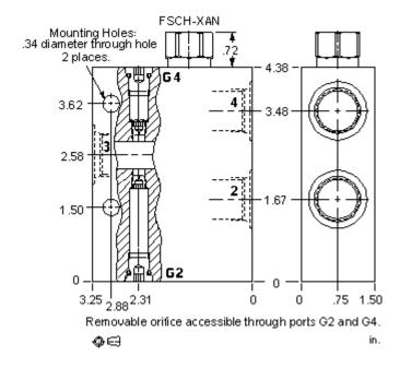
This valve assembly is intended for use in tractive systems. It incorporates a divider/combiner valve along with provisions for slip orifices. The divider/combiner provides 2 equal flows for positive traction and the slip orifices can be sized to allow for steering.
