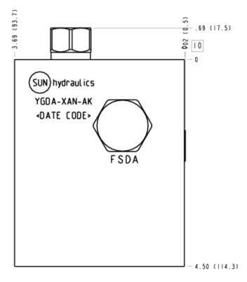
This valve assembly uses 3 divider/combiner valves to provide 4 equal bidirectional flows. In the dividing mode, flow coming into AB is divided into 4 equal flows, A1, A2, B1, B2. In the combining mode the assembly throttles the 4 flows coming into A1, A2, B1, B2 keeping them equal.
