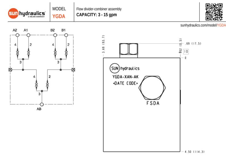
This valve assembly uses 3 divider/combiner valves to provide 4 equal bidirectional flows. In the dividing mode, flow coming into AB is divided into 4 equal flows, A1, A2, B1, B2. In the combining mode the assembly throttles the 4 flows coming into A1, A2, B1, B2 keeping them equal.
