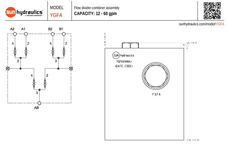
This valve assembly uses 3 divider/combiner valves to provide 4 equal bidirectional flows. In the dividing mode, flow coming into AB is divided into 4 equal flows, A1, A2, B1, B2. In the combining mode the assembly throttles the 4 flows coming into A1, A2, B1, B2 keeping them equal.
