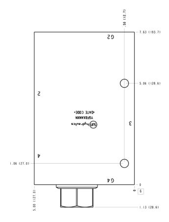
This valve assembly is intended for use in tractive systems. It incorporates a divider/combiner valve along with provisions for slip orifices. The divider/combiner provides 2 equal flows for positive traction and the slip orifices can be sized to allow for steering.
