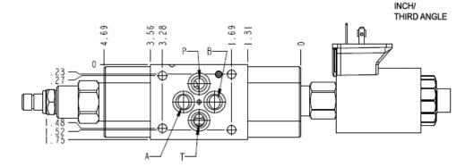
This assembly consists of a pilot-operated pressure reducing/relieving valve with a separate drain (port 4) which reduces a high primary pressure at the inlet (port 2) to a constant reduced pressure at port 1, with a full-flow relief function from port 1 to tank (port 3). Draining the pilot section
