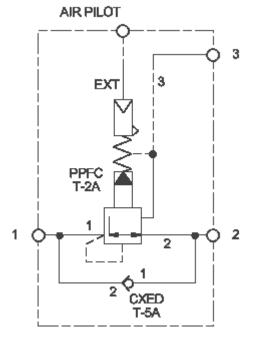
This assembly consists of a pilot-operated pressure reducing/relieving valve which reduces a high primary pressure at the inlet (port 2) to a constant reduced pressure at port 1, with a full-flow relief function from port 1 to tank (port 3). A reverse flow check allows free flow from port 1 to port 2. The air signal is supplied through a port in the hex-end of the cartridge and the hydraulic setting is directly proportional to the air setting at a ratio of 20:1 (hydraulic:air).
