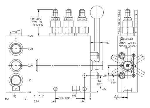
Pilot-operated, balanced-piston relief cartridges are normally closed pressure regulating valves. When the pressure at the inlet (port P) reaches the valve setting, the valve starts to open to tank (port T), throttling flow to regulate the pressure. These valves are accurate, have low pressure rise vs. flow, they are smooth and quiet, and are moderately fast. This assembly includes 3 relief valves which allows the selection of 3 separate pressure settings plus an all ports blocked position.
