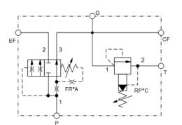
This assembly consists of a bypass/restrictive, fixed-orifice, priority flow control which takes an input flow at port P and uses it to satisfy the priority flow at port CF. If the input flow exceeds the priority flow requirement, the excess is bypassed out port EF. The bypass flow may be used in a secondary circuit. The relief valve protects the controlled flow from over-pressurization, relieving excess flow out of port T.
