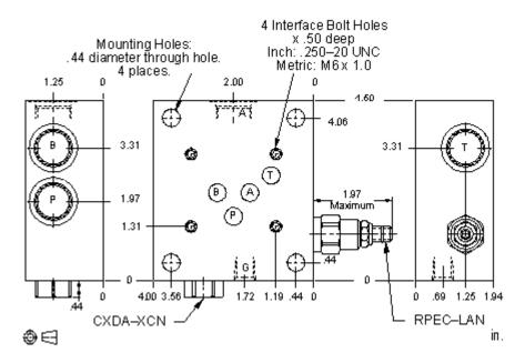
This assembly consists of a 30 PSI check and a pilotoperated, balanced-piston relief cartridge which is a normally closed pressure regulating valve. When the pressure at the
