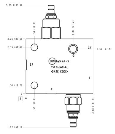
This assembly consists of a bypass/restrictive, fixed-orifice, priority flow control which takes an input flow at port P and uses it to satisfy the priority flow at port CF. If the input flow exceeds the priority flow requirement, the excess is bypassed out port EF. The bypass flow may be used in a secondary circuit. The relief valve protects the controlled flow from over-pressurization, relieving excess flow out of port T.
