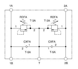
This assembly provides cross-port relief and anti-cavitation protection between ports 1 and 2.
