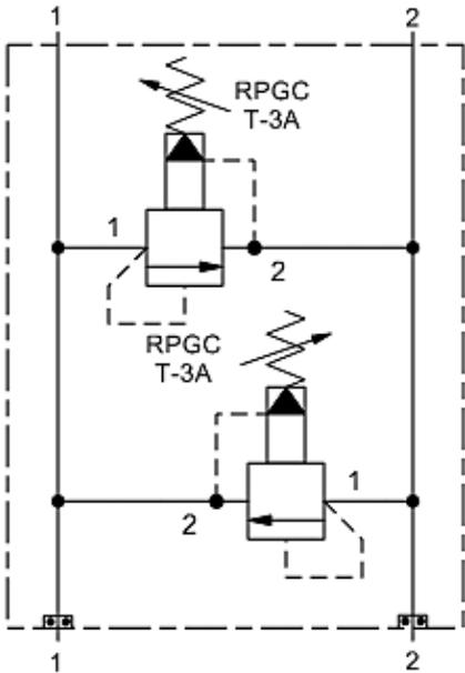
This assembly provides cross-port relief protection between ports 1 and 2.
