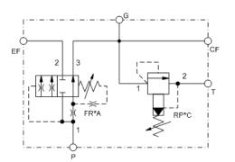
This assembly consists of a bypass/restrictive, fixed-orifice, priority flow control which takes an input flow at port P and uses it to satisfy the priority flow at port CF. If the input flow exceeds the priority flow requirement, the excess is bypassed out port EF. The bypass flow may be used in a secondary circuit. The relief valve protects the controlled flow from over-pressurization, relieving excess flow out of port T.
