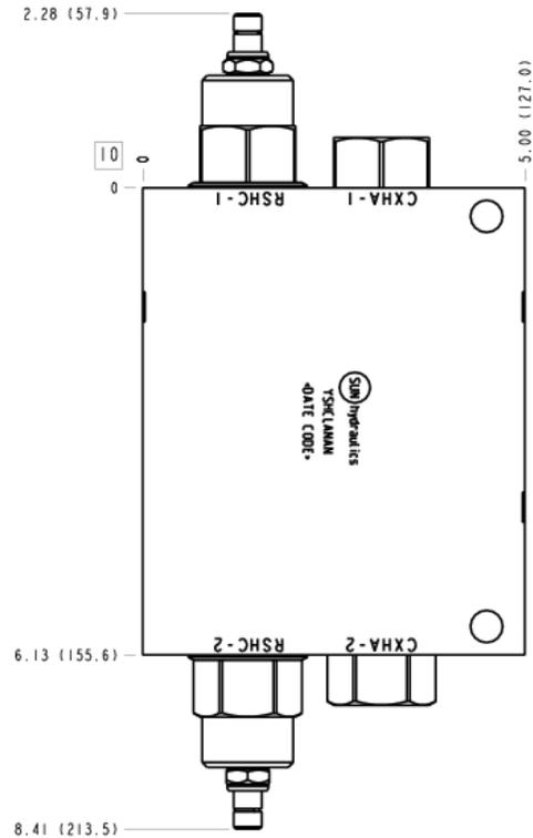
This assembly consists of dual pilot-operated, balanced piston sequence valves, each with a separate reverse flow check. It can be used to sequence the operation of two cylinders.
