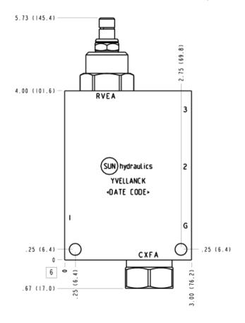
This assembly consists of a 30 PSI check and a pilot-operated, balanced-piston relief cartridge which is a normally closed pressure regulating valve. When the pressure at the inlet (P port) reaches the valve setting, the valve starts to open to tank (T port), throttling flow to regulate the pressure. These valves are accurate, have low pressure rise vs. flow, they are smooth and quiet, and are moderately fast.
