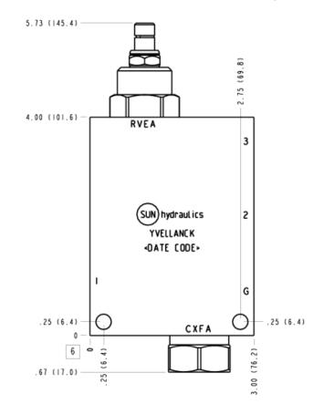
This assembly consists of a 30 PSI check and a pilot-operated, balanced-piston relief cartridge which is a normally closed pressure regulating valve. When the pressure at the inlet (P port) reaches the valve setting, the valve starts to open to tank (T port), throttling flow to regulate the pressure. These valves are accurate, have low pressure rise vs. flow, they are smooth and quiet, and are moderately fast.
